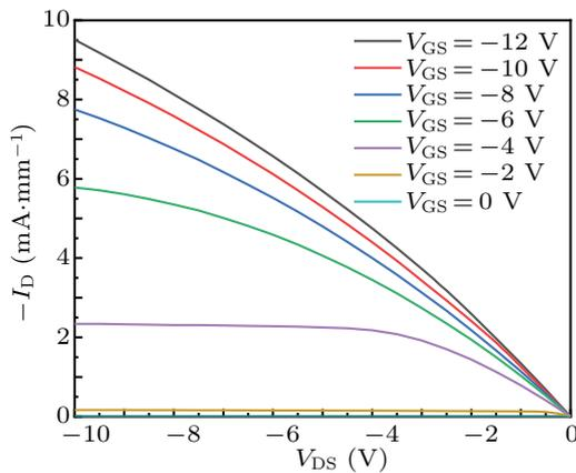
**Fig. 7.** Output characteristics of the E-mode p-GaN-MOSFET. The doping concentration of p-GaN is set as  $9.5 \times 10^{16} \text{ cm}^{-3}$ .
