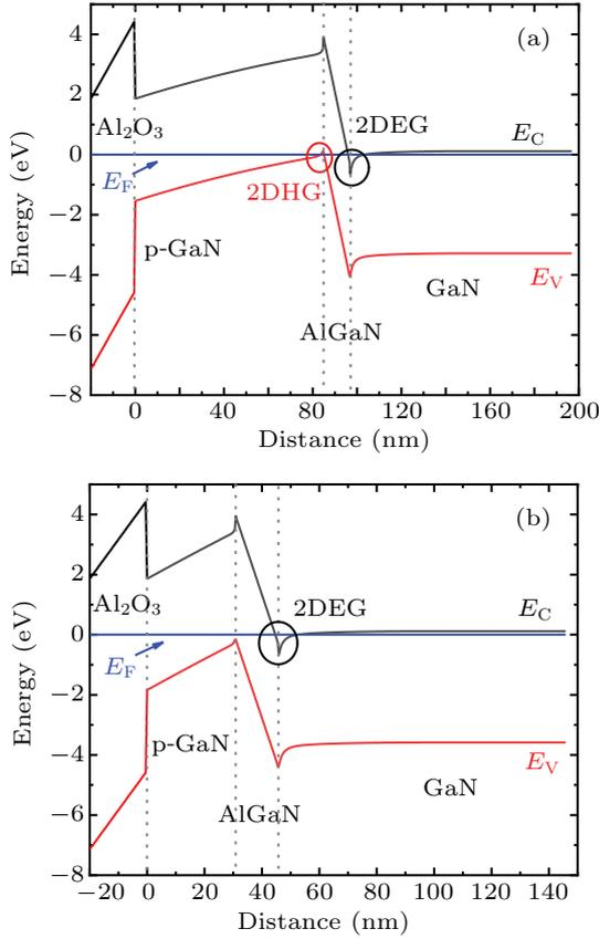
**Fig. 2.** The simulated band diagrams of a structure with an oxide/p-GaN/AlGaIn/GaN. It is clearly visible that the thickness of p-GaN in panels (a) and (b) are 85 nm and 31 nm, respectively.
