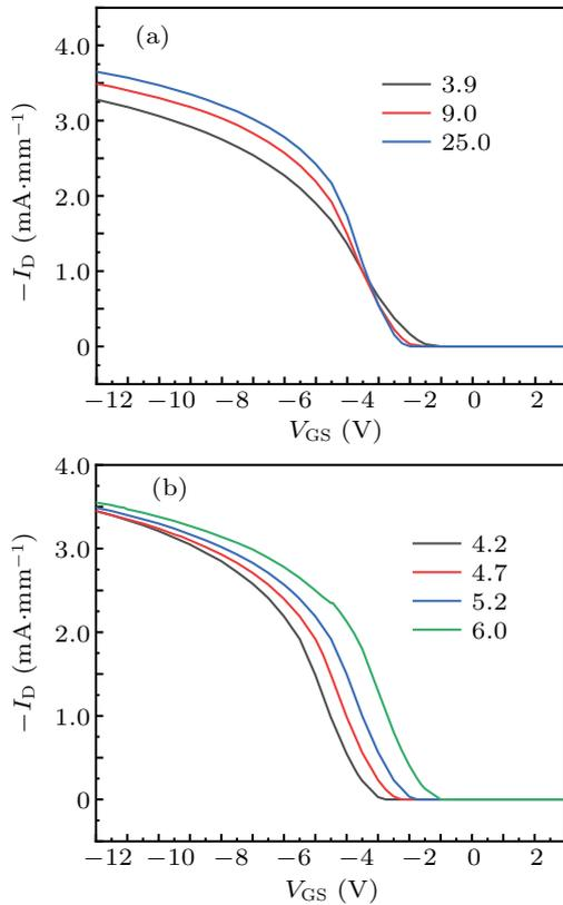
**Fig. 6.** Transfer characteristics of the E-mode p-GaN-MOSFET with various (a) gate dielectric relative permittivities and (b) gate metal work-functions.
