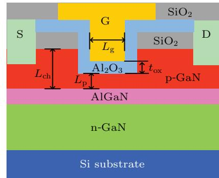
Fig. 1. Cross-section of the recessed-gate E-mode p-GaN/AlGaIn/GaN MOSFET.
