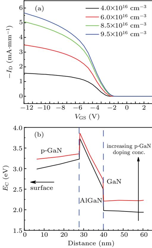
**Fig. 4.** Transfer characteristics of the E-mode p-GaN-MOSFET with various  $N_p$  from  $4.0 \times 10^{16} \text{ cm}^{-3}$  to  $9.5 \times 10^{16} \text{ cm}^{-3}$ . (b) The simulating band diagram of p-GaN/AlGaN/GaN structure.
