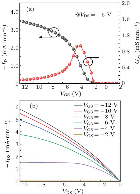
**Fig. 3.** (a) Transfer and (b) output characteristics of the E-mode p-GaN-MOSFET. The doping concentration of p-GaN is set as  $6.5 \times 10^{16} \text{ cm}^{-3}$ .
