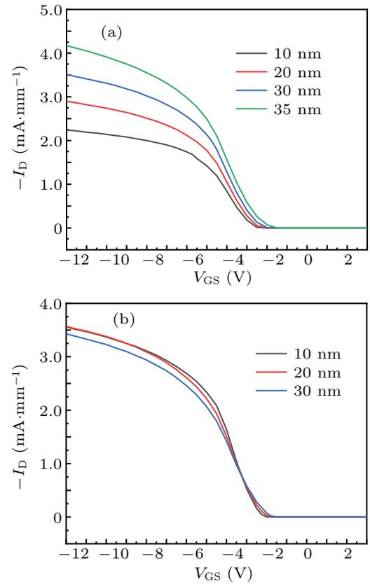
**Fig. 5.** Transfer characteristics of the E-mode p-GaN-MOSFET with various (a) p-GaN layer thicknesses under the gate and (b)  $\text{Al}_2\text{O}_3$  thicknesses under the gate.
