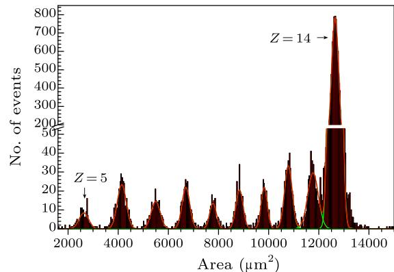
**Fig. 3.** Base-area distribution of etched tracks of 736 A MeV  $^{28}\text{Si}$  and their fragments in CR-39 detector after C target.
