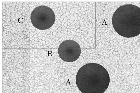
**Fig. 2.** Tracks of charged particles on CR-39.
