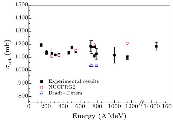
**Fig. 4.** Dependence of the total charge-changing cross sections on the energy.
