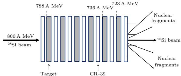
**Fig. 1.** The typical configuration of the stacks for this experiment.
